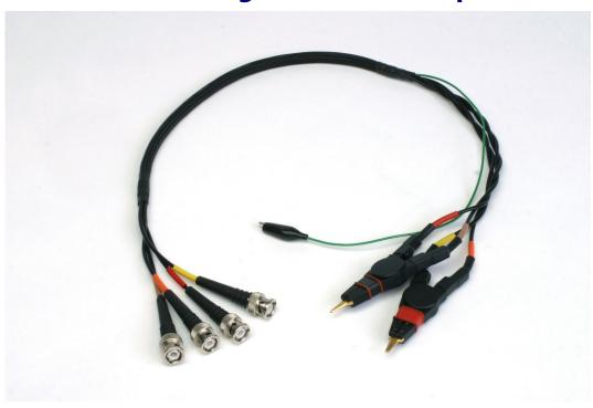
Wayne Kerr Kelvin Clips consist of a 0.6 m cable assembly terminated with four BNC connectors at the analyzer end and a pair of 4-terminal Kelvin clips at the Device Under Test end.
