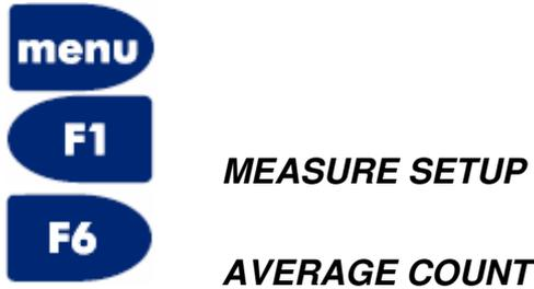
Select the required number of average count (1 to 99) by using the numeric keyboard and when finished press **ent** and you will return to the main menu.
